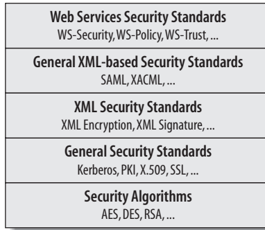
FIGURE 14-3 . Security stack for XML and Web Services
